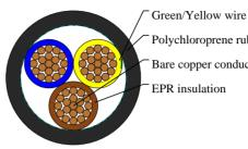
Polychloroprene rubber outer jacket Bare copper conductor
